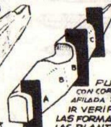
FILAR CON CORTA-PLUMAS AFILADA Y LIJA FINA, IR VERIFICANDO LAS FORMAS CON LAS PLANTILLAS
